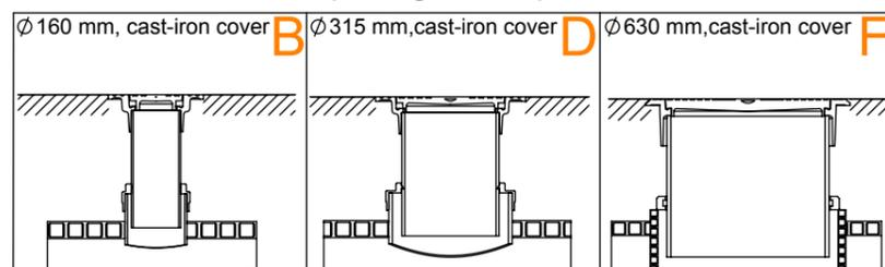
Service opening height : standard height 950 mm  or h=..... mm
